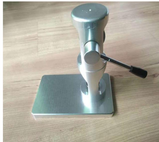
**The press** allows the pan to be sealed very easily. Under the pressure of the plunger the pan is cold welded hermetically with the lid. After changing plunger and die you can use the press for other crucibles.
